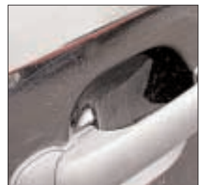
Multiple light scratching in a localised area where neither primer nor metal is exposed
