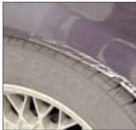
Significant scratching which exposes bare metal or primer
