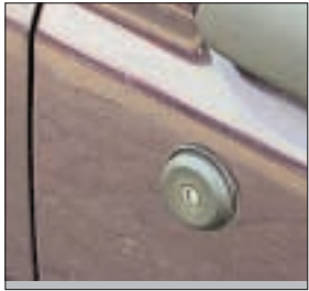
Excessive chipping of paintwork around door-lock (caused by driver negligence)
