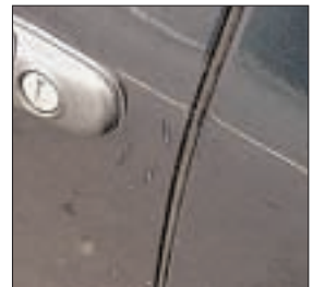
Isolated scratches under 50mm in length
