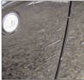
Multiple scratches in a localised area where bare metal or primer is exposed
