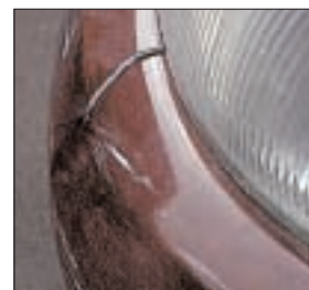
Bumpers or rubbing strips that are cracked, broken, missing or severely misshapen
