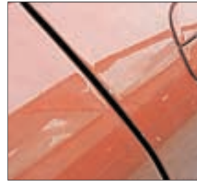
Light chipping of door edge or surround
