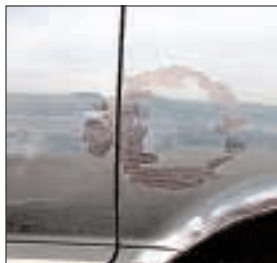
Inadequate retouching or repair work
