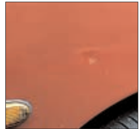
Isolated dents under 45mm in diameter
