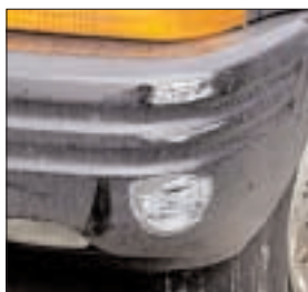
Bumper with excessive scuffing
