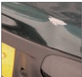
Any dent where bare metal or primer is exposed
